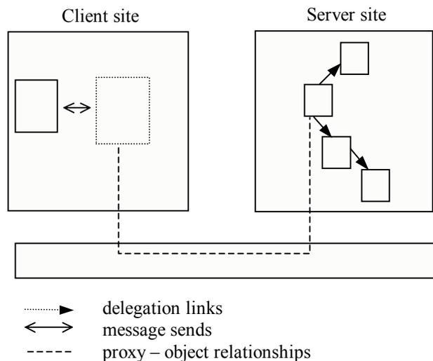
Figure 3. The client side sees a single object. The delegation machinery is hidden on the server's side.
