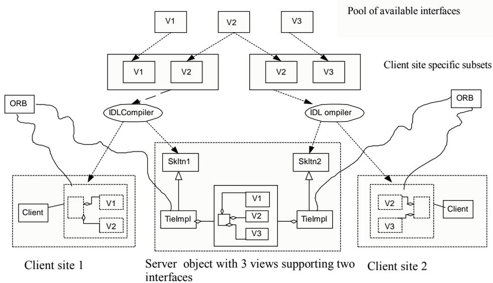
Figure 6. Server Object(s) implement several client interfaces.
